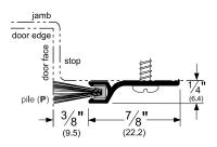
A (Mill Finish Aluminum) BDG (Bright Dip Gold Anodized Aluminum) D (Dark Bronze Anodized Aluminum) **G** (Gold Anodized Aluminum) PW (Painted White Aluminum)
