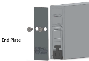
Figure 4 - Properly Installed End Plate
